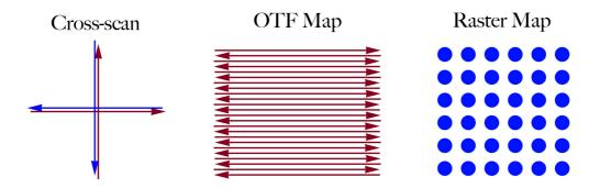
In the case of cross-scan, a subscan is a single arrow (a line across the target), four arrows – i.e. two full crosses – constitute the schema which might be repeated as many times as needed within the scan. For OTF maps, the subscan is again the single arrow, and the scan coincides with the whole map obtained with lines along one axis only (e.g. along RA or Dec). For raster maps, which are based on discrete acquisitions, each point is a subscan, and the final map constitutes the scan.
